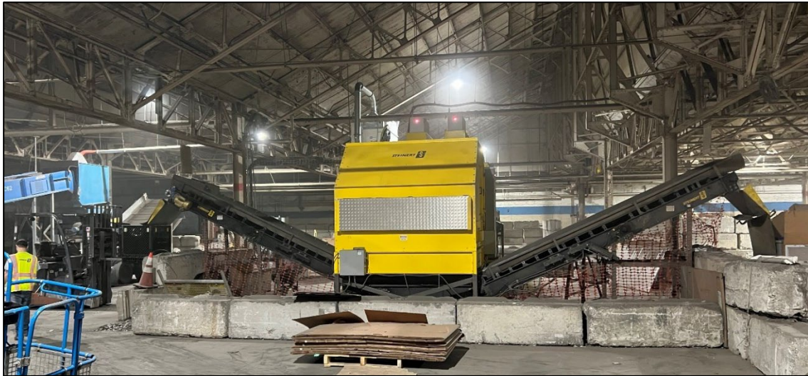
Figure 3 – Steinert Multi-Sensor Sorter Testing Oracle Ridge Samples
