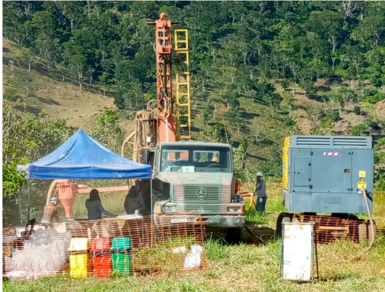
Figure 6: RC drill rig drilling at the Rio Negro prospect.
