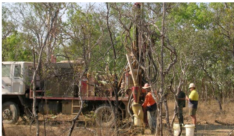
Figure 1: Air core drill rig on black soil plain
