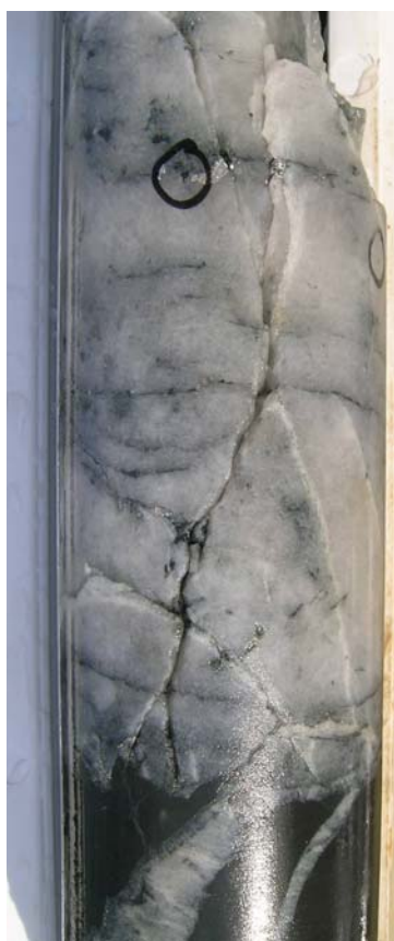
Specks of visible gold (inside circles) with arsenopyrite in quartz vein, Glencoe drill hole GLD001: 86.4m
