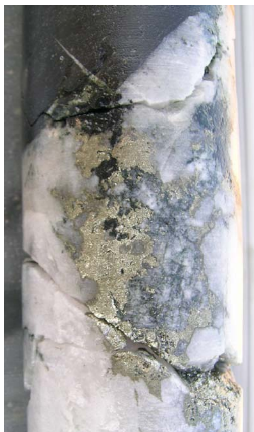
Pyrite-arsenopyrite aggregate in quartz vein GLD001: 68.1m
