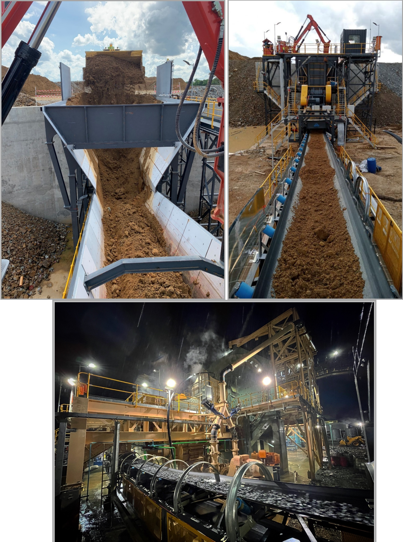
Figure 7 | Crushed ore conveyed to the stockpile
