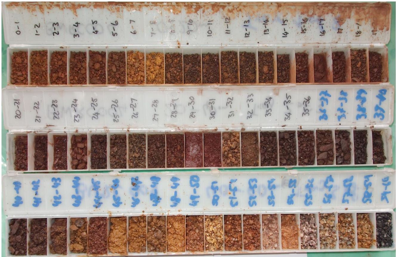
Figure 3. Drill hole BWRC004; 48m @ 38.30 % Fe, 40.20 % SiO 2 , 0.051 %P from surface
