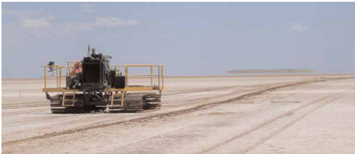
Air core drilling on Lake Way
