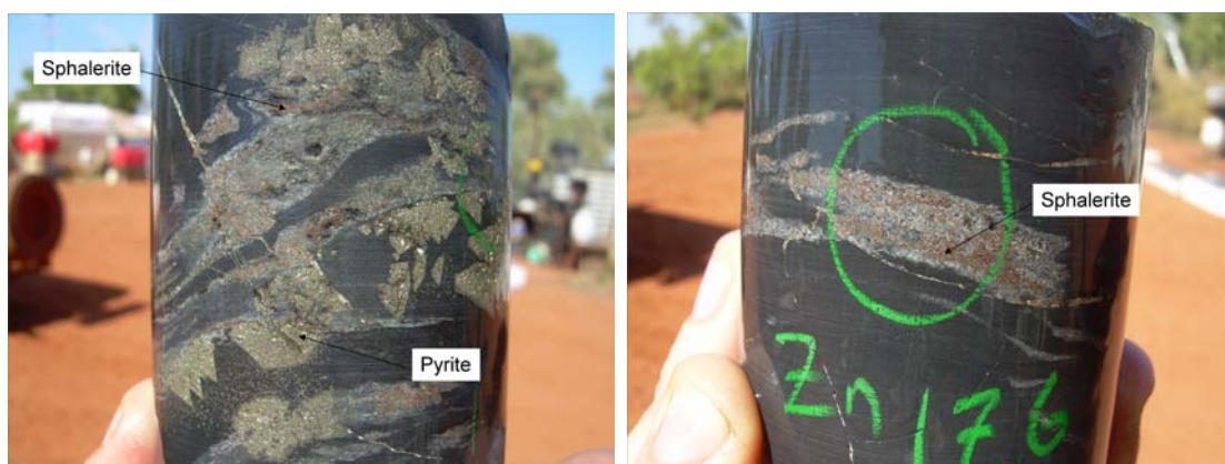
Photo 1 and 2: EPT0799 - Examples of base metal sulphide veins at BM2
