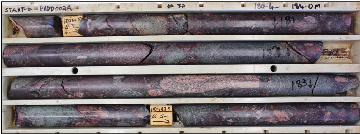
Photo 1: PADD002A 180.4m to 184.0m – Hematite-altered, polymictic breccia containing clasts of felsic porphyry, gneiss and mafic igneous rocks
