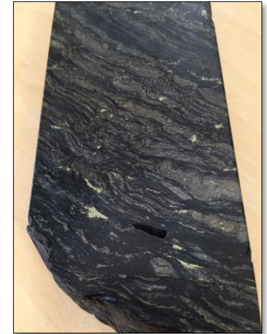
Disseminated chalcopyrite in carbonaceous shale EPT 2282 ~259.2m downhole (1.0%Cu)
