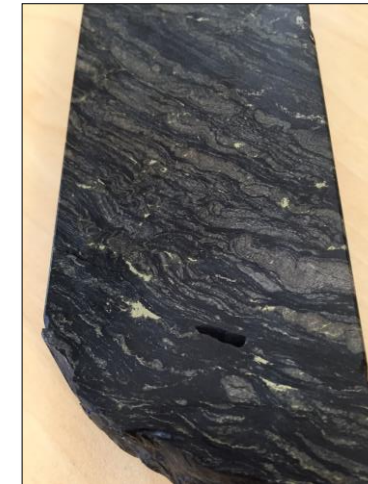
Disseminated chalcopyrite in carbonaceous shale EPT 2282 ~259.2m downhole (1.0% Cu)
