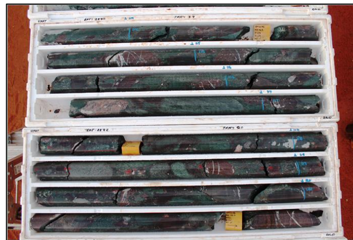
Drill core from Aria IOCG-style intrusion with copper sulphides (EPT2276)
