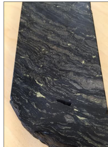
Lookout Rocks (Zambian Copperbelt analogue): Disseminated chalcopyrite in carbonaceous shale ~259m down hole (1.0%Cu) (EPT2282)
