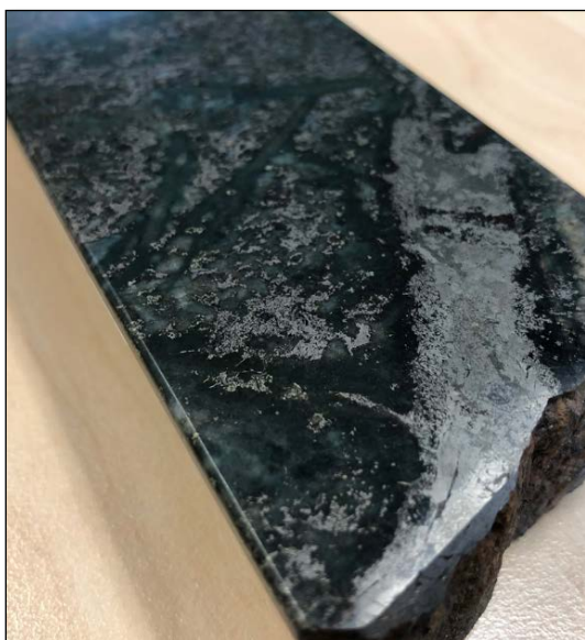
Photo 1 (L) – LSPC-3 (Newmont, 1980s) ~44m. Veins and disseminations of pyrrhotite and minor chalcopyrite within an altered calcareous sediment.
