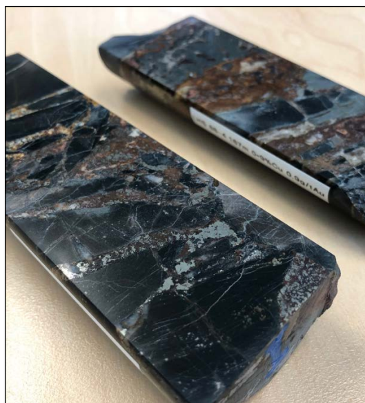
Photo 1 (L) – LSPC-3 (Newmont, 1980s) ~44m. Veins and disseminations of pyrrhotite and minor chalcopyrite within an altered calcareous sediment.
