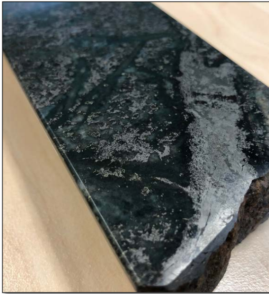
Photo 2 (L) – LSPC-3 (Newmont, 1980s) ~44m. Veins and disseminations of pyrrhotite and minor chalcopyrite within an altered calcareous sediment.
