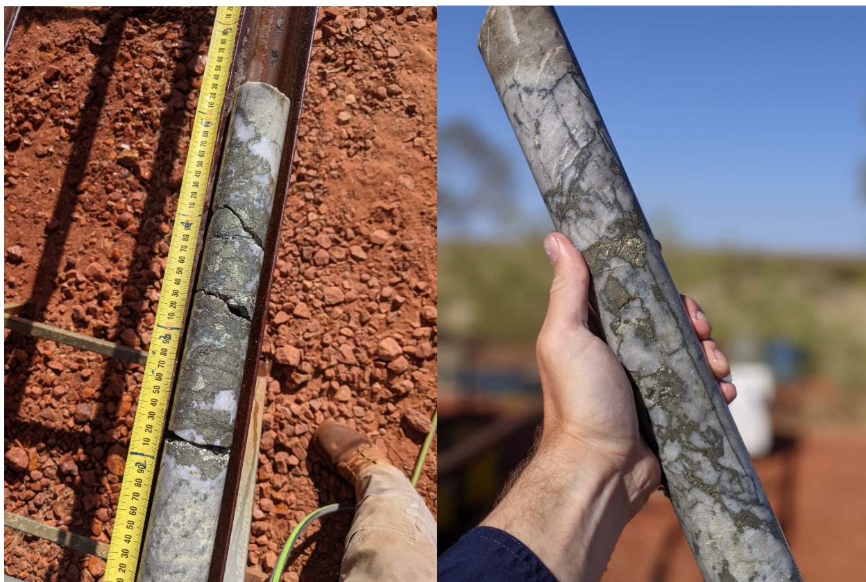
Photo 4 – Example of semi-massive pyrite/chalcopyrite ~ 347m in ETG0243
