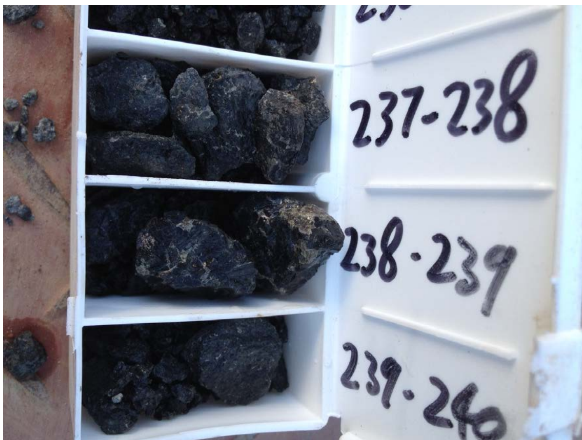
Plate 4. Drill chips, hole PLRC003, Interval 237-240m
