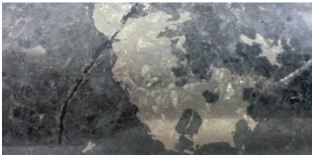
PLRC003, at 337.4 metres Downhole Niton XRF on Sulphides: 5.5% Ni, 1.5% Cu
