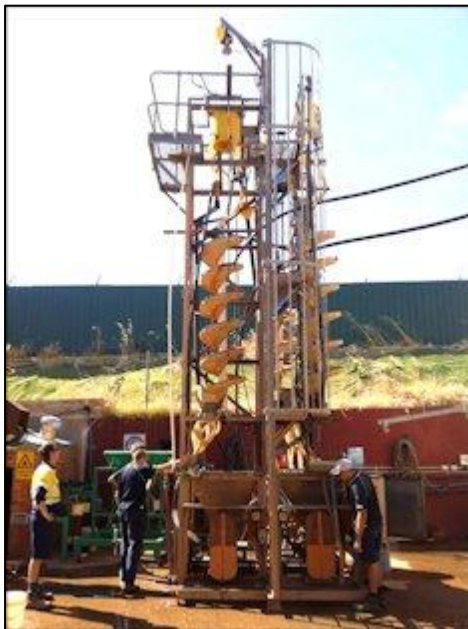
Figure 2 – Gravity separation testwork under way at AML Pty Ltd in Perth
