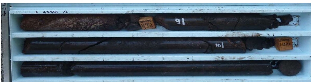
Photograph 1. Massive MnO mineralisation in ADD006 (8.90m to 12.00m) Significant intersection of brecciated and massive (>50% MnO) manganese mineralisation.
