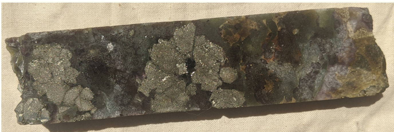
Figure 6: Sample lvt-21-14 of pyritic fluorite from 33.44m
