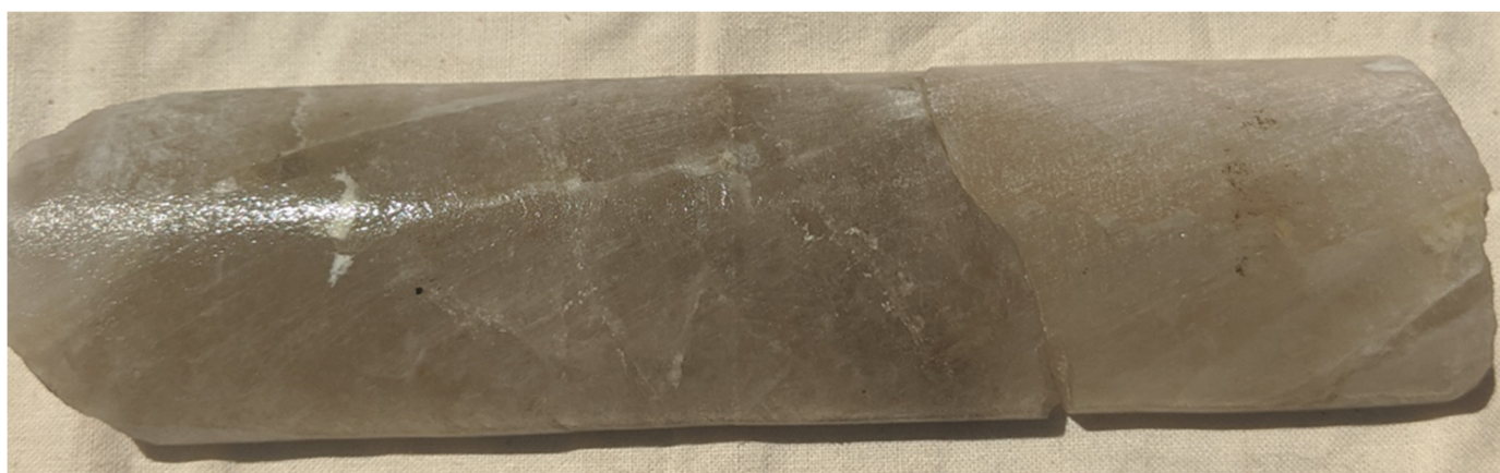
Figure 4: Sample IVT-21-6 of Cryolite from 20.15m.
