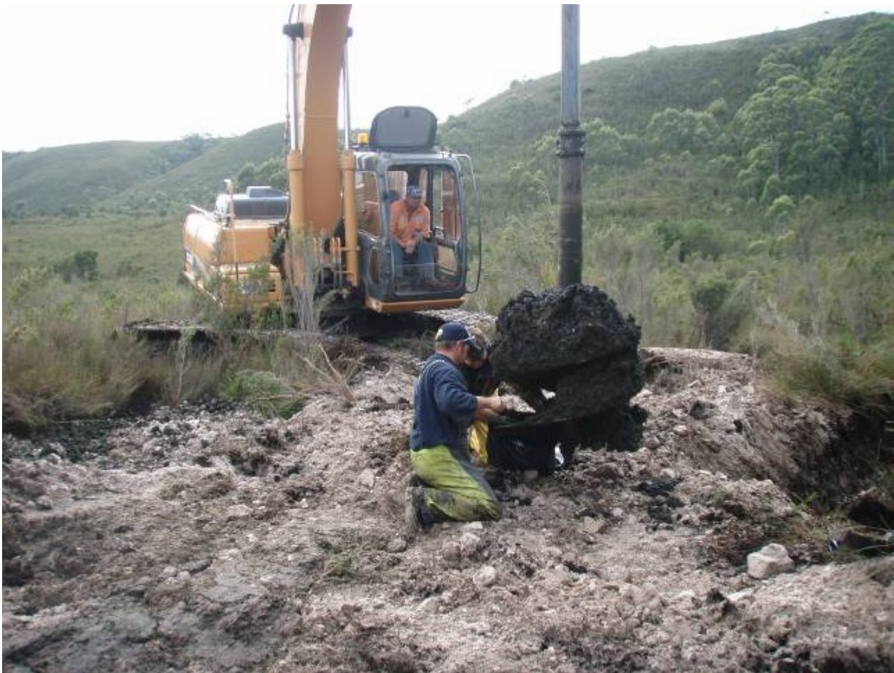
Figure 2: Large diameter auger sampling of zinc-in-peat, Grieves Siding, Professor Project, Western Tasmania.
