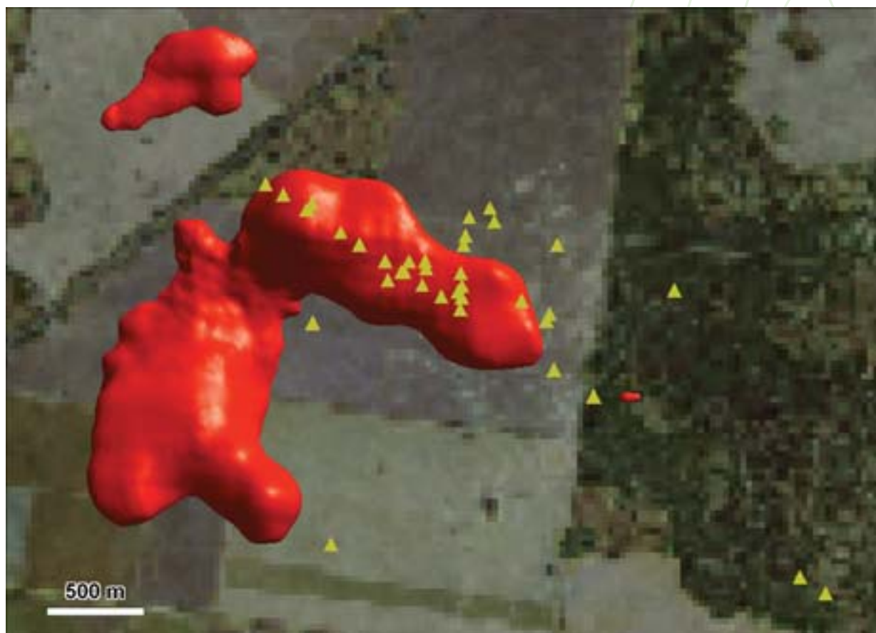
Figure 3. Chargeability anomalies from a recent 3D IP survey at Tara tin project central NSW indicating large areas of untested mineralisation (Δ indicates drill collar)
