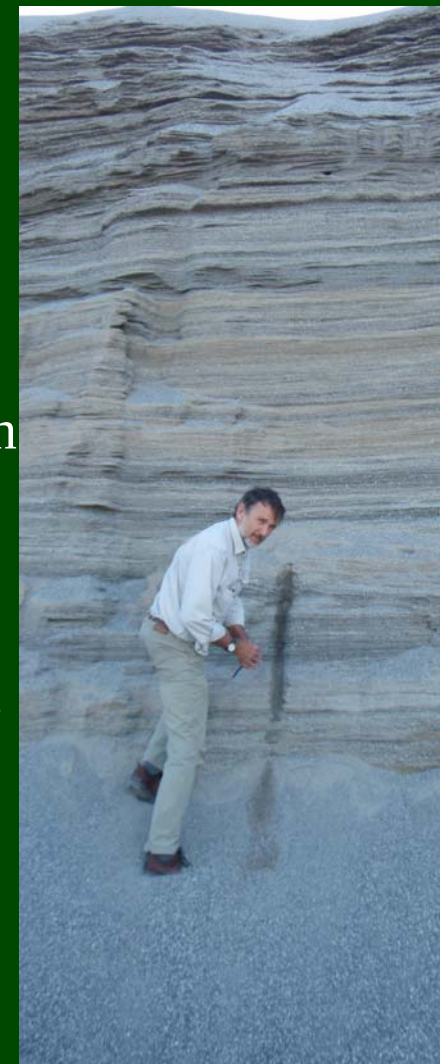
Mt Carbine tailings. These are expected to form a significant resource, with ~1M cubic metres grading at ~0.1% \text{WO}_3 per tonne.
