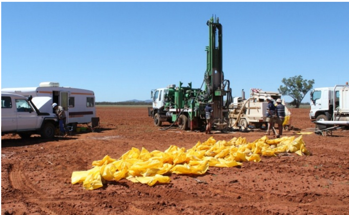
Tara Tin Project – Drill-testing placer tin targets, March-April 2010.
