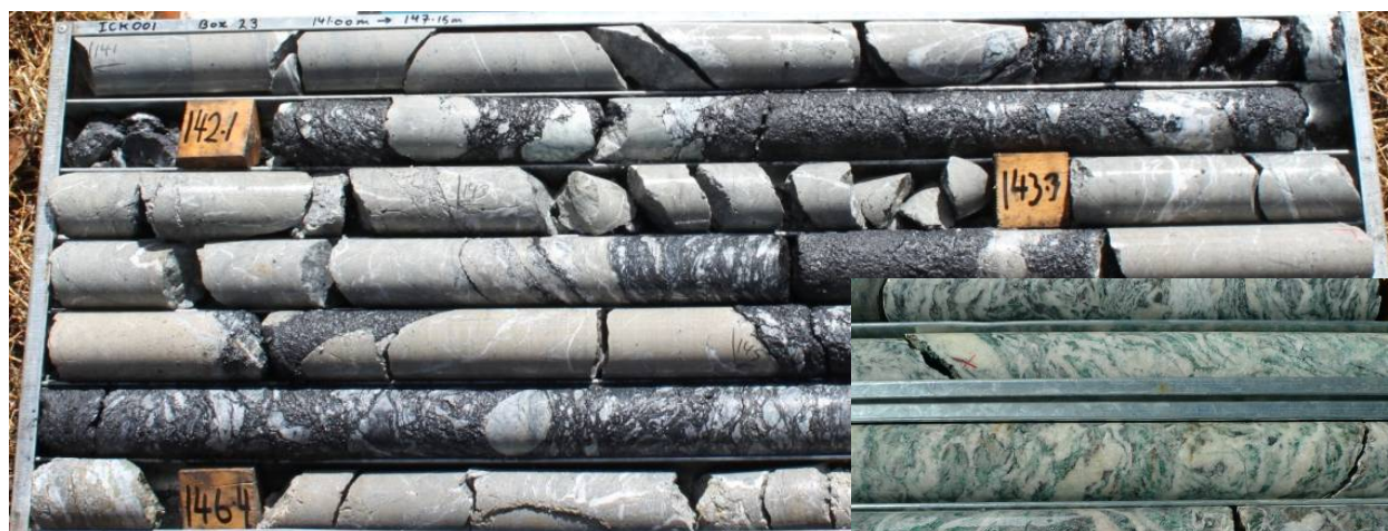
Highly altered / mineralised dyke and graphitic breccia zones within the 8m zone from 140m depth in drillhole ICK-001 grading 1.27g/t gold (above), and adjacent listwanite alteration (left)
