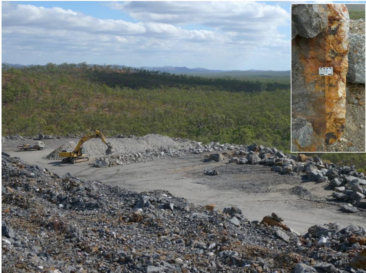
Bulk sampling of mineralised waste ahead of pilot ore-sorter trials scheduled to commence in August 2010. Inset shows mineralised boulder from the waste stockpile.
