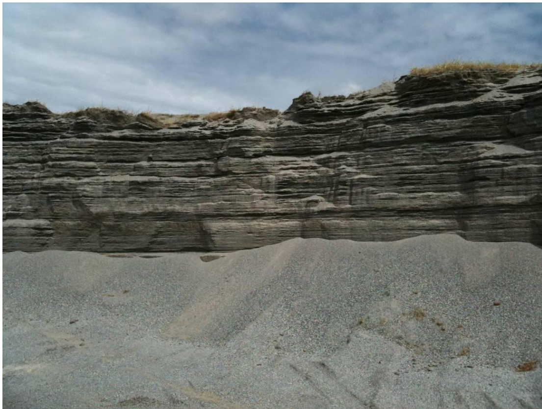
Mt Carbine Tailings, largest particle size is 8mm with the majority of the Wolframite and Scheelite in the fines
