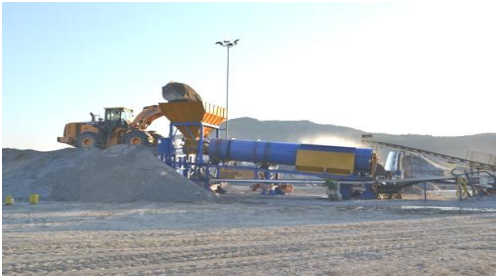
Carbine Tungsten Limited Tailings Retreatment Plant: newly installed scrubber at work.
