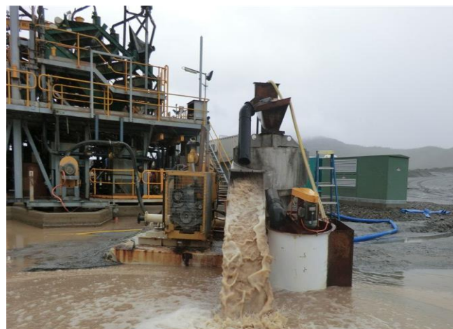
Testing of Ultra Fines Centrifuge recovering tungsten particles down to three micron.
