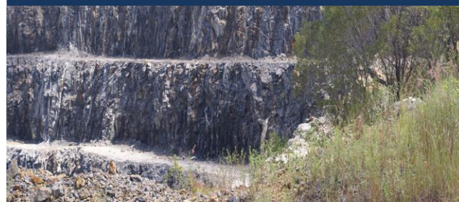
Mt Carbine Tungsten Deposit – vertical, sub-parallel, quartz Veins hosting wolframite and scheelite mineralization.
