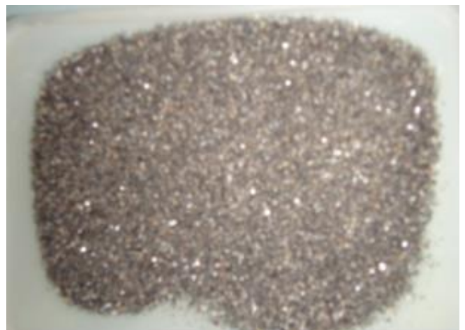
Medium -1mm + 0.3mm jigging concentrate under natural light.
