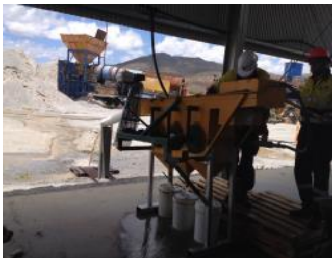
Jig Test Work – Tailings Retreatment Operation
