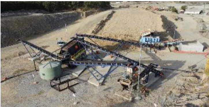
Stage 1 Crushing and Screening Circuit in production
