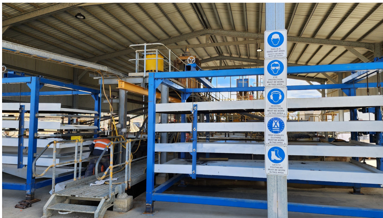
Figure 6: Eight additional shaker tables have been installed and commissioned to increase processing capacity.
