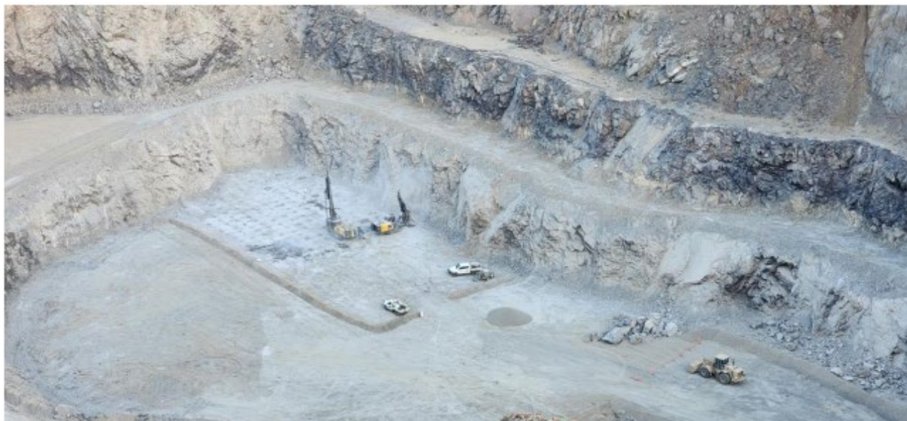
Figure 27: Orana Drill and Blast Rigs working on the holes for the first calibration blast.
