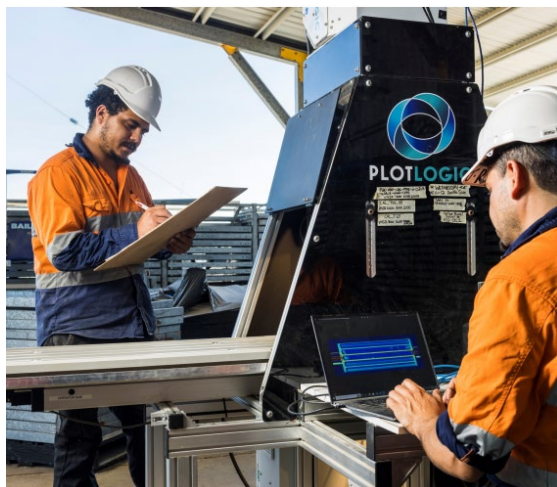
Figure 12: Plot Logic sensor, scanning drill core.
