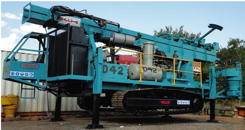
Figure 5: Wallis Drilling tracked RC drill after conversion at Mayoko
