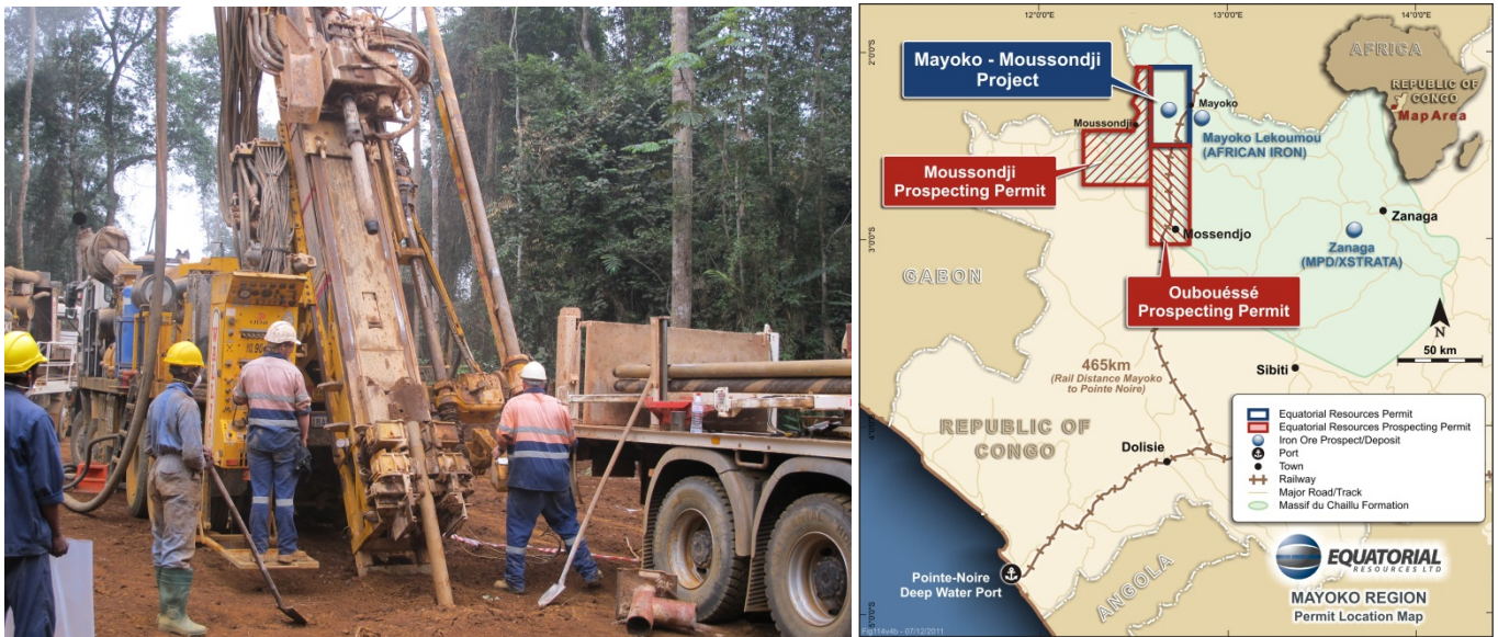
Figure 3 & 4: RC drill rig in operation at Makengui Prospect; Mayoko-Moussondji Project Location Map
