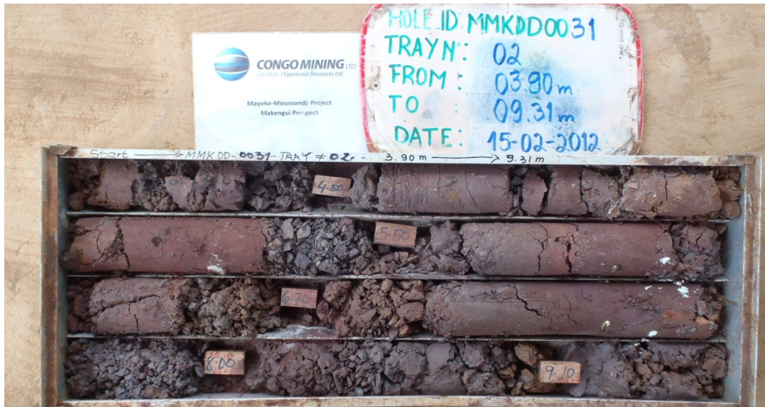
Figure 6: Enriched Hematite - PQ Metallurgical Hole from Mayoko-Moussondji (awaiting assay)
