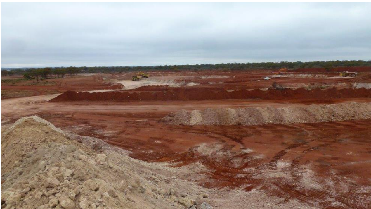
Initial mining and preparing the first bench at Penny's Find Gold Mine
