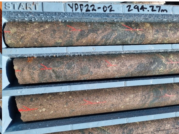
Figure 2 – YDD22-02 Massive pyrrhotite with blebby pyrite and patchy disseminated chalcopyrite
