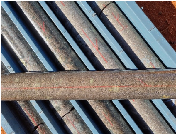
Figure 1 – YDD22-02 Massive pyrrhotite with disseminated blebby chalcopyrite and globules of pyrite rimmed by chalcopyrite @299.7m
