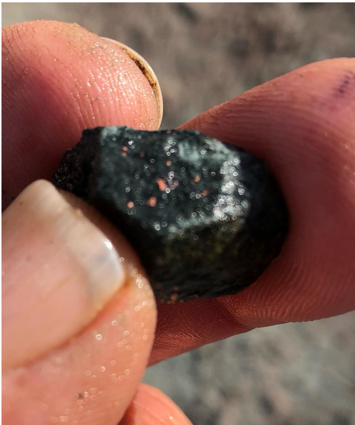
Photo 4. Traces of speckly native copper on rock chip surface from YRC26-20 (89m to 90m)
