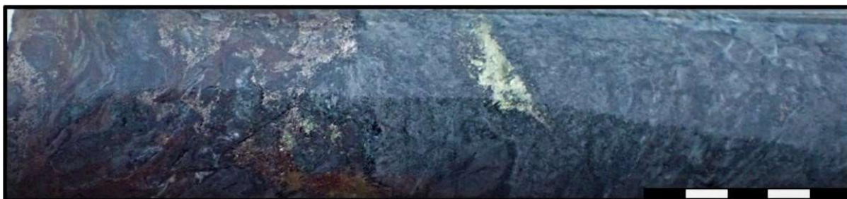
Picture 4: Drill core from KIODD002 (92.7m) – blebs of pyrrhotite-sphalerite-chalcopryite hosted in quartz-chlorite-actinolite altered volcanic siltstone.
