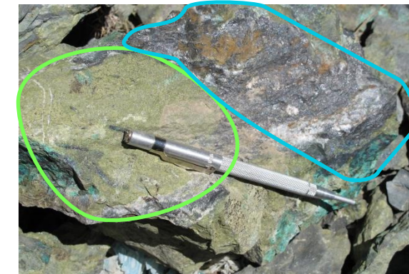
Rock sample at Luna; the blue polygon shows the disseminated bornite throughout the rock matrix. The green ellipse shows the large epidote altered clast. This photo demonstrates the potential that ore has at Luna to be 'easily' separable from the gangue under relatively coarse crushing.
