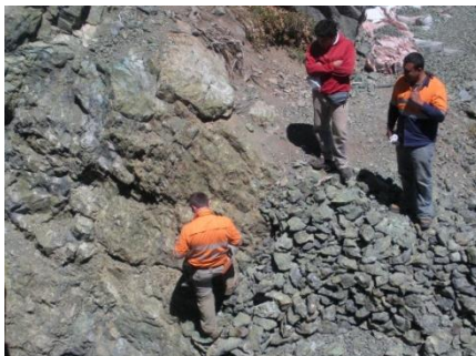
Mapping and sampling at Alto del Valle located within Luna; mineralised breccia's are situated within faults and feature strong epidote & chlorite alteration which provides a good rock 'signature' to explore for further occurrences.
