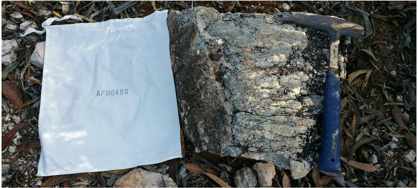
Figure 10. Photo of the AP00460 sample site, which returned 1.89% Li 2 O. The greenish hewed material on the right hand 80% of this sample contains abundant spodumene. This specimen was taken from an historic costean. ‡
