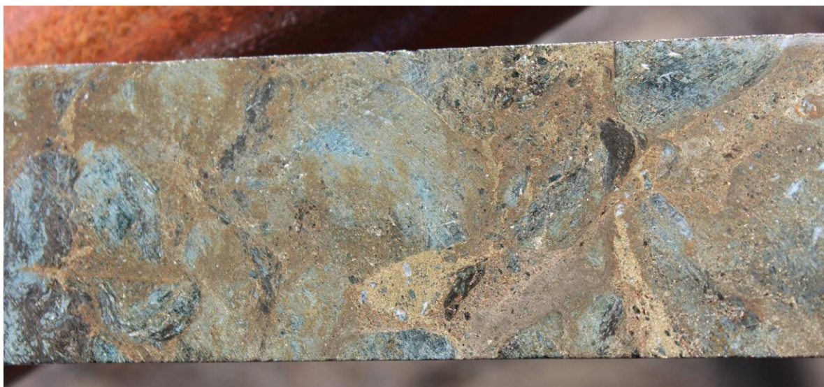
Figure 6. Nickel sulphides in drill core from Spargoville.
