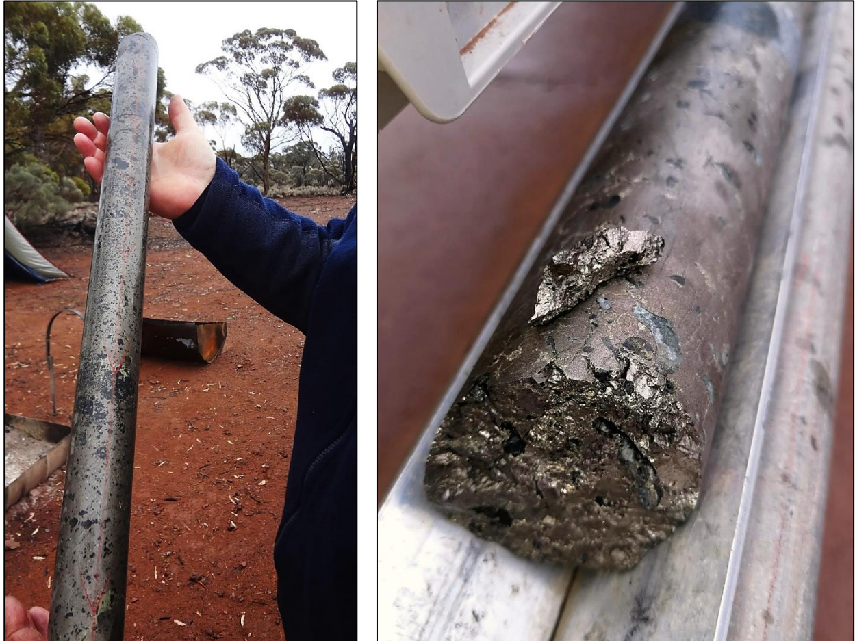
Figure 2. Ni-Cu bearing massive sulphide zone in diamond drill hole CBDD030 drilled 300m south of the T5 Ni-Cu discovery zone (436.7m-437.6m shown).
