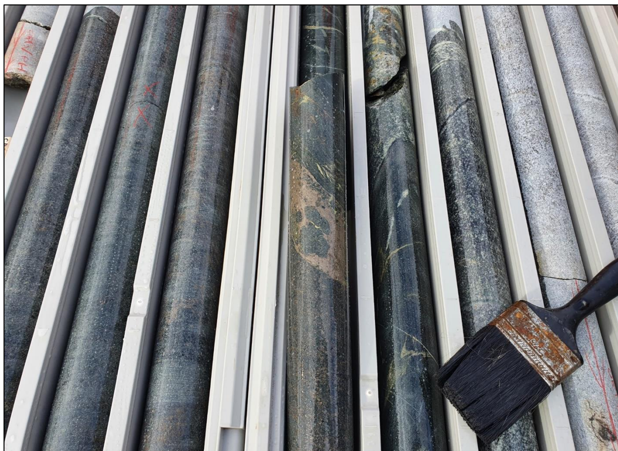
Figure 6. Anomalous Ni-Cu-PGE bearing sulphides in diamond drill hole CBDD028 at the T5 Ni-Cu discovery zone (161m-169m shown).
