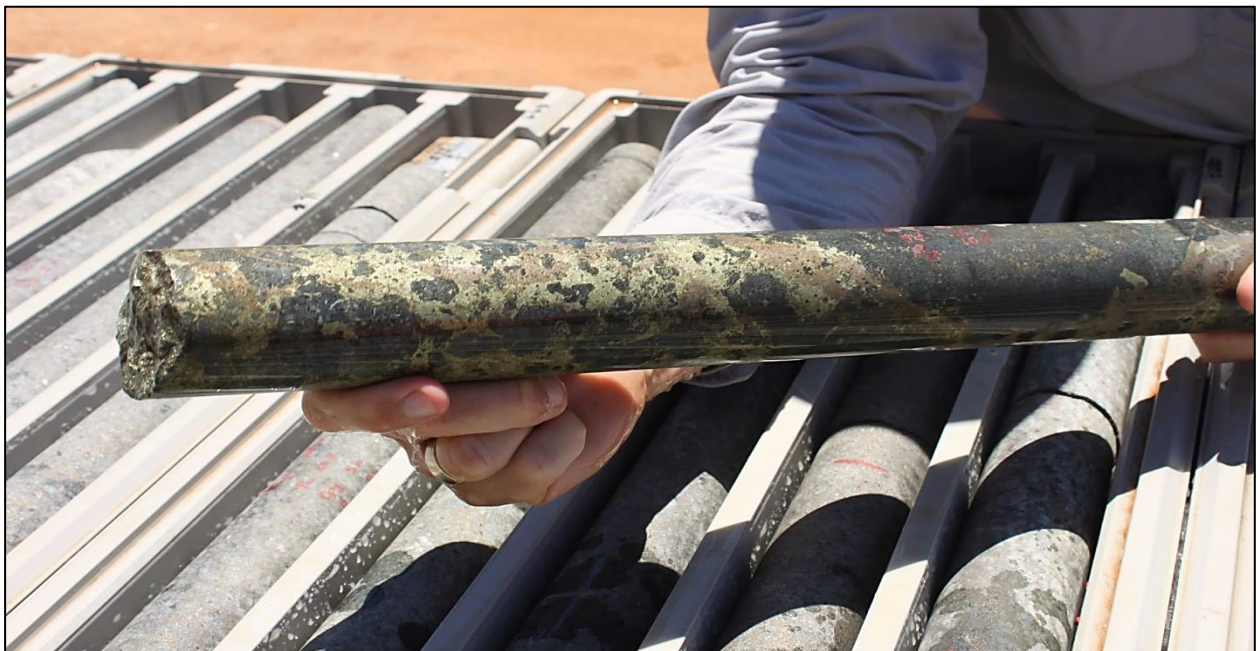
Figure 1. Copper rich breccia sulphide zone (chalcopyrite+pyrrhotite+pentlandite) within drill hole CBDD033 which returned 0.78m at 5.45% Cu, 1.17% Ni, 19.30g/t Ag & 0.74g/t PGE's from the T5 Prospect, Carr Boyd Rocks Project (387.2m-387.8m shown).
