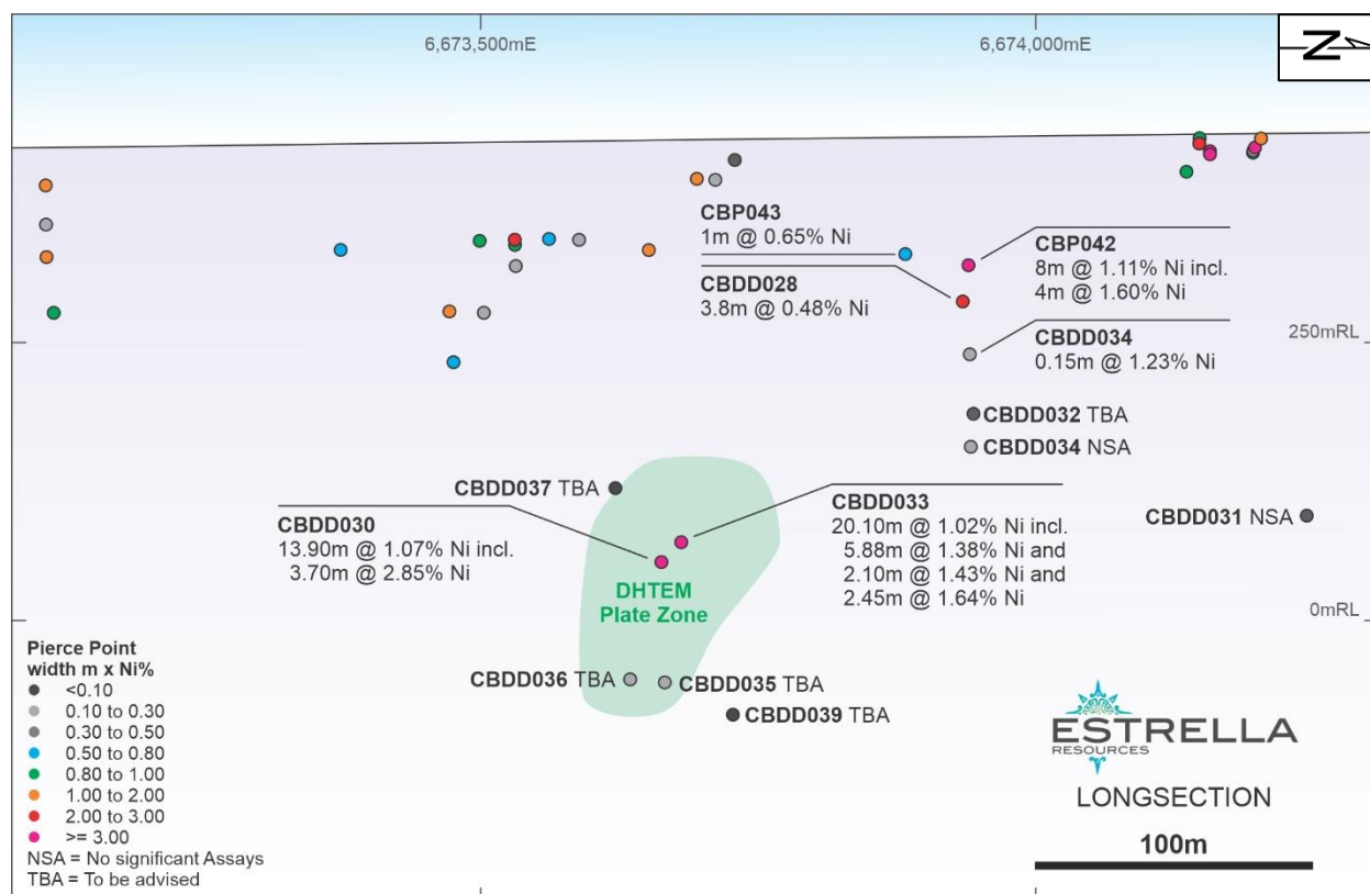
Figure 2. Longsection (looking west) along the T5 Prospect Zone showing shallow historical pierce points into the basal contact which are coloured by intersection-width (m) x Ni% grade. Recent drilling by Estrella is labelled and details are tabulated in Tables 1-3. The DHTEM anomaly plate area from recent survey work is shown by the green zone.
