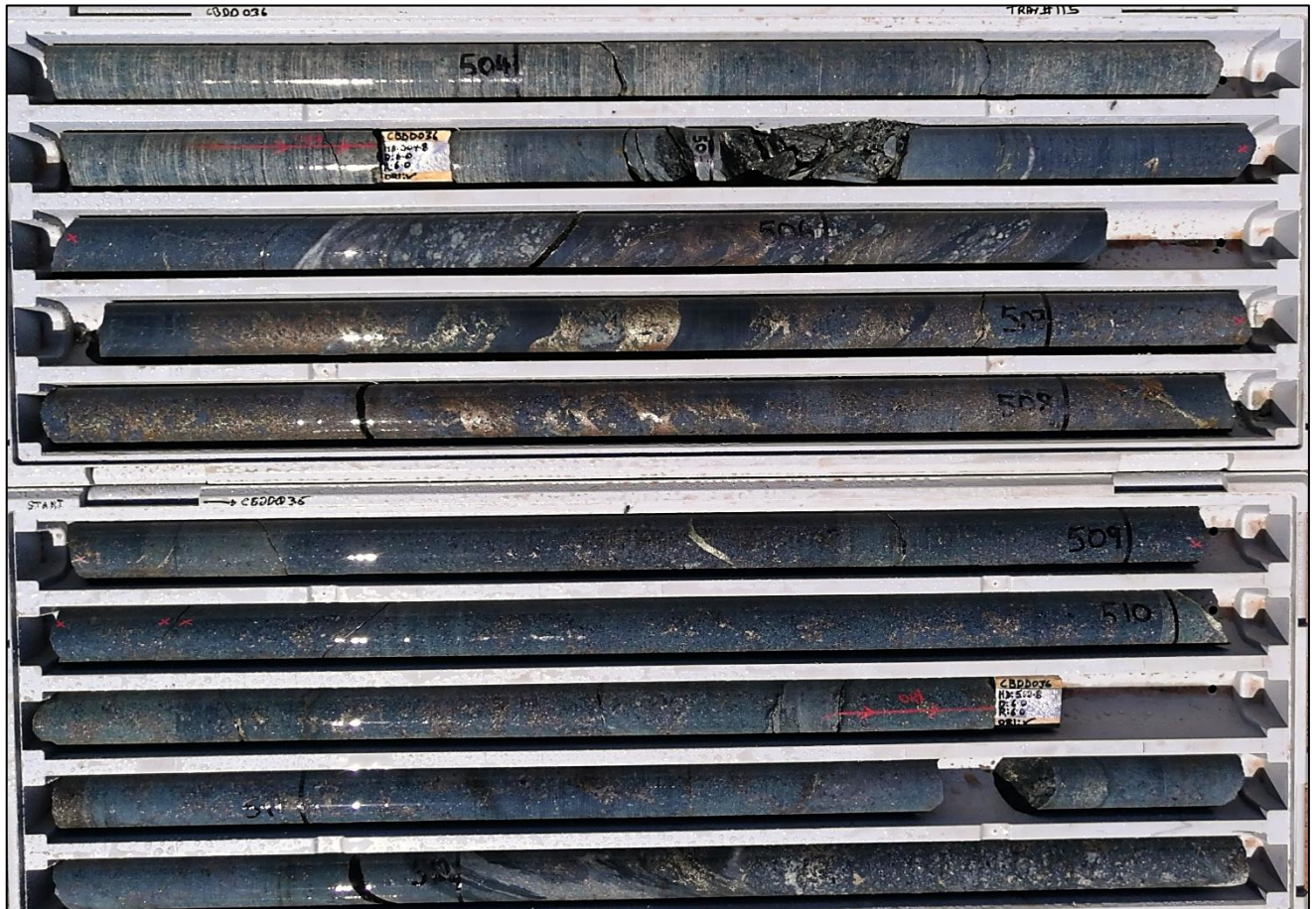
Figure 6. Ni-Cu bearing disseminated, matrix and stringer/vein sulphides within diamond drill hole CBDD036 at the T5 Ni-Cu discovery (503.6m- 512.5m shown).
