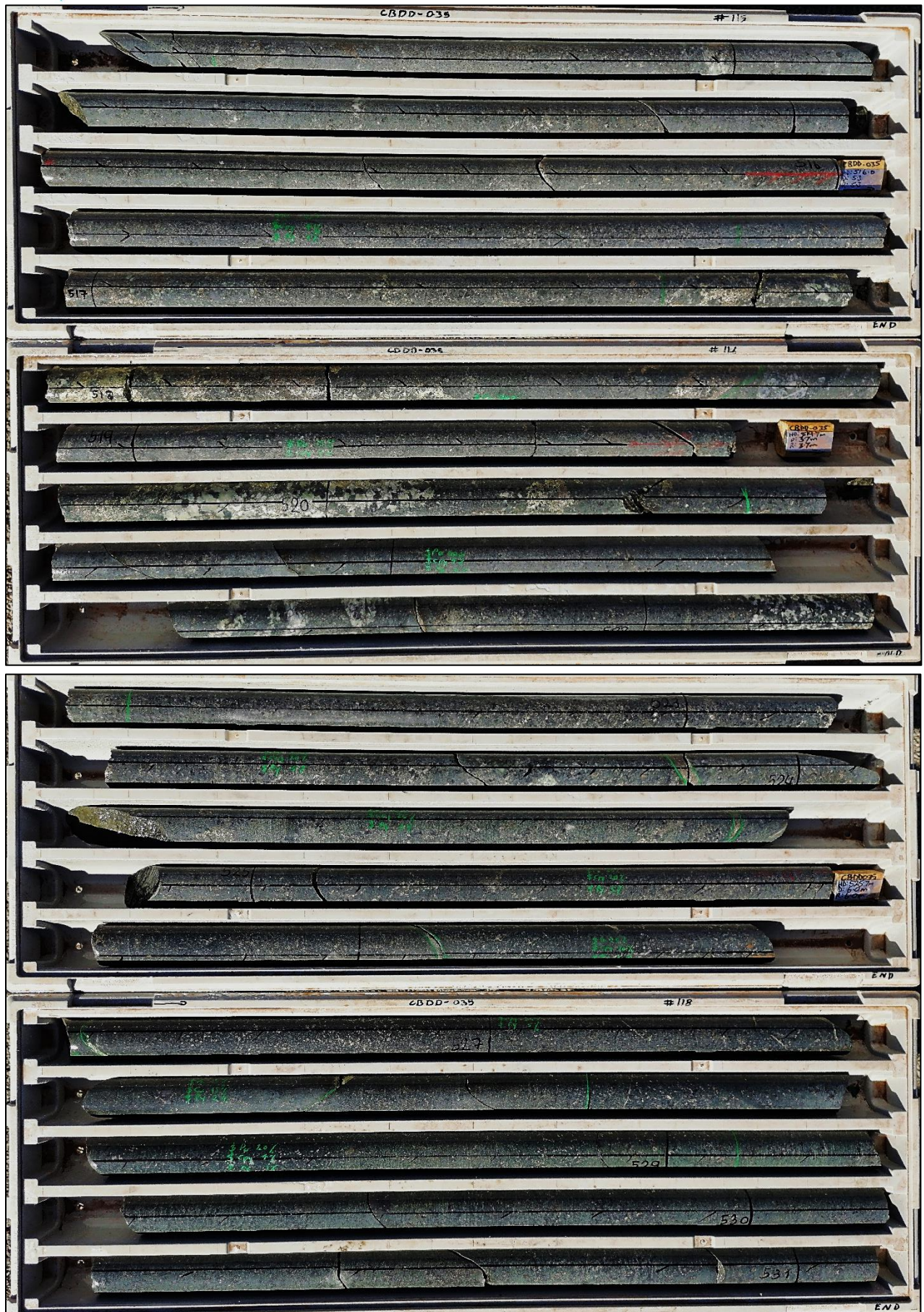
Figure 5. Ni-Cu bearing disseminated, matrix and stringer/vein sulphides within diamond drill hole CBDD035 at the T5 Ni-Cu discovery (513.3m- 531.1m shown).
