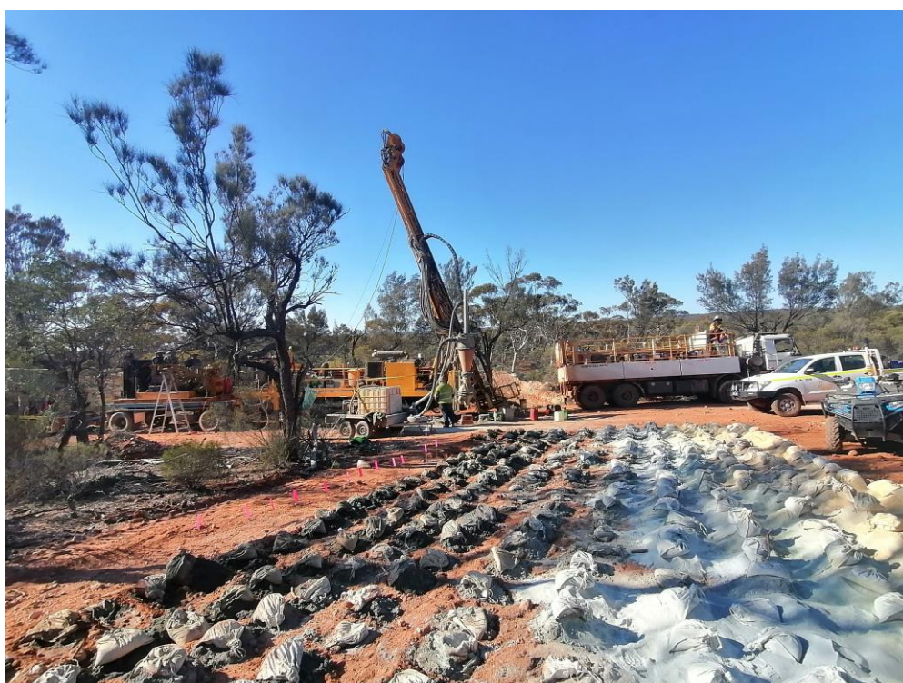
Figure 5: TDA Multipurpose RC Diamond Rig drilling CBP076.
