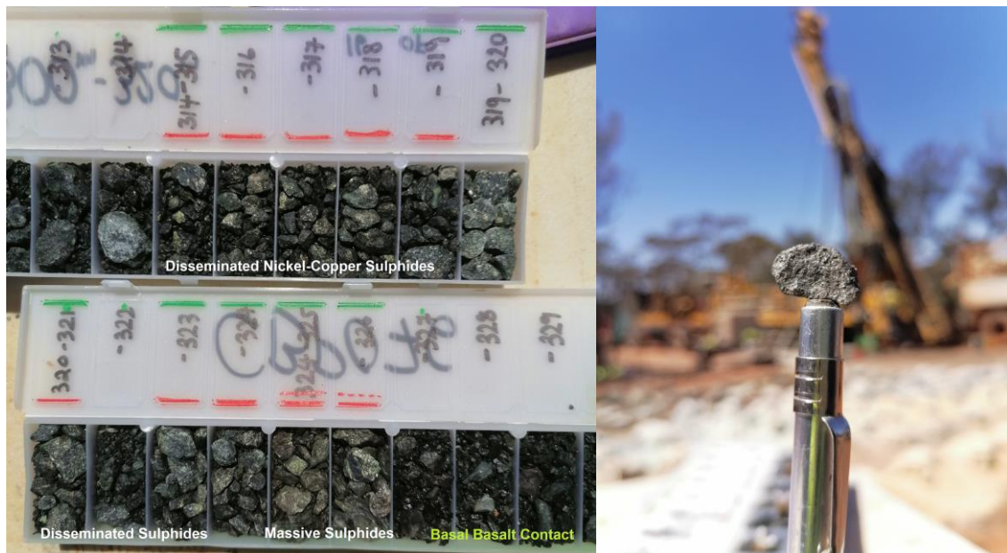
Figure 1: Disseminated and basal massive nickel-copper sulphides in CBP076.
