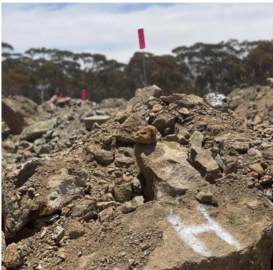
Figure 2: Bulk sample stockpile R24 prior to crushing, located on the 5B ROM Pad, containing 5% violarite and 25% nickel and iron oxides. Assays are pending analysis.
