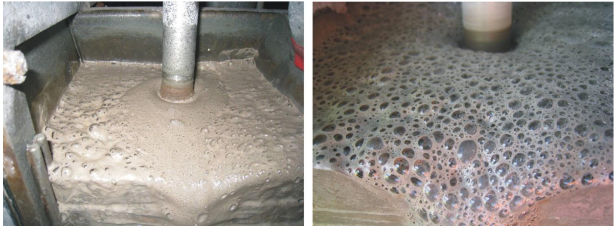
Figure 3. The REE-phosphate cleaner cell (left), and a close-up of the REE-phosphate mineral froth.
