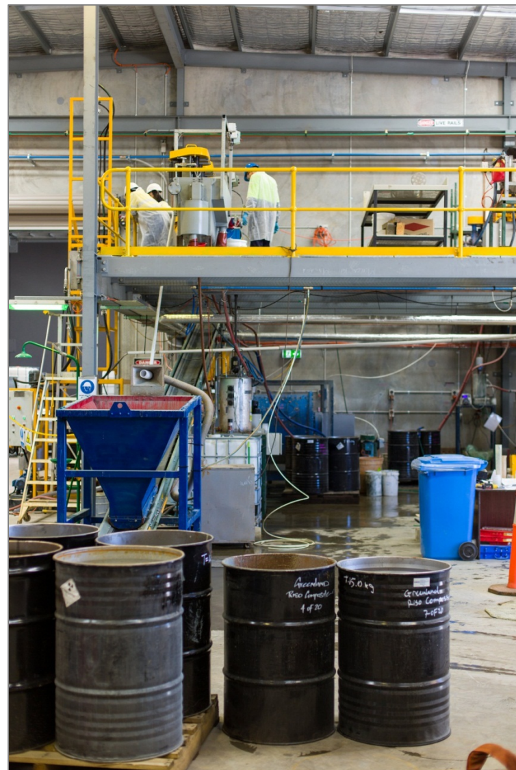
Continuous pilot plant operation at SGS Laboratories, Perth, produced outstanding results; >300kgs of concentrate produced
