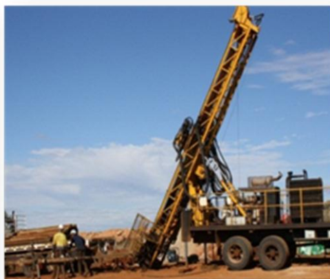
Diamond Core Drilling
