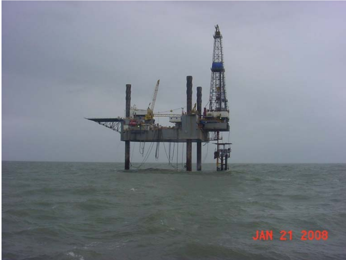
A picture of the Hercules 152 rig positioned over the "B" Platform and drilling Pompano SL 103229 # 1 Well through the 36" caisson.
