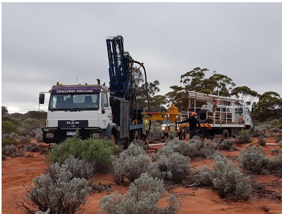
Figure 4: Aircore drilling now underway at Gimlet
