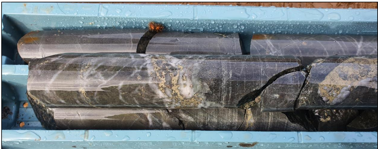
Figure 4: A chlorite-epidote altered chalcopyrite sulphide quartz vein overprinting potassic biotite-magnetite veins from 322m in Hole 4
