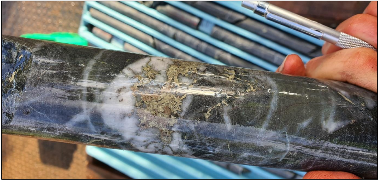
Figure 3: Chalcopyrite + Pyrite + Quartz veins from Hole 4 @ 322.5m.
