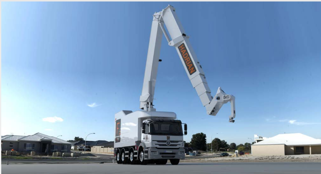
Figure 1 – The Hadrian X will be a road-capable, truck-mounted machine with a folding 30m boom
