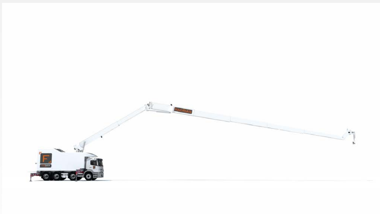
Figure 4 - Full extension of the Hadrian X's 30m boom, allowing it to 3D print a complete brick structure, course by course
