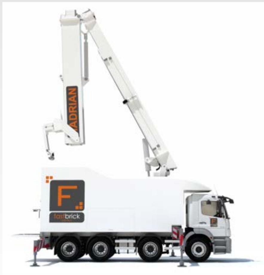
The Hadrian X bricklaying robot
