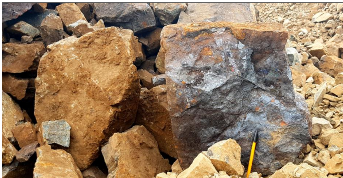
Figure 5 – Typical massive magnetite being exposed on the floor of the mining pits first bench. These contain visible sulphides have been assayed and shown to contain copper.
